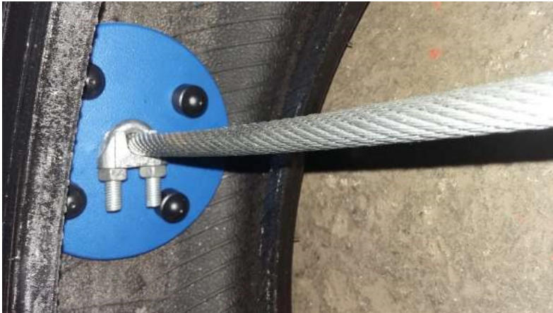
LEFT: Detail of single cable grip on inside of tyre
