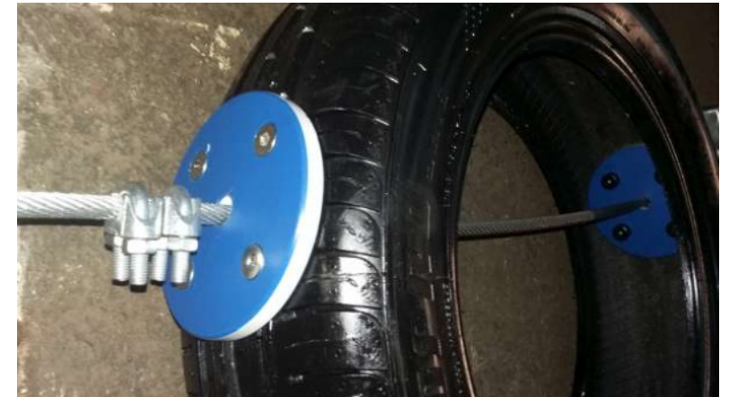
RIGHT: Detail of two cable grips on outside of tyre
